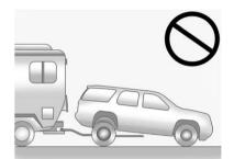
*Notice:* Towing the vehicle from the rear could damage it. Also, repairs would not be covered by the vehicle warranty. Never have the vehicle towed from the rear.
